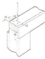
Back head - Screwed and glued to jamb and front head at the end of the installation
